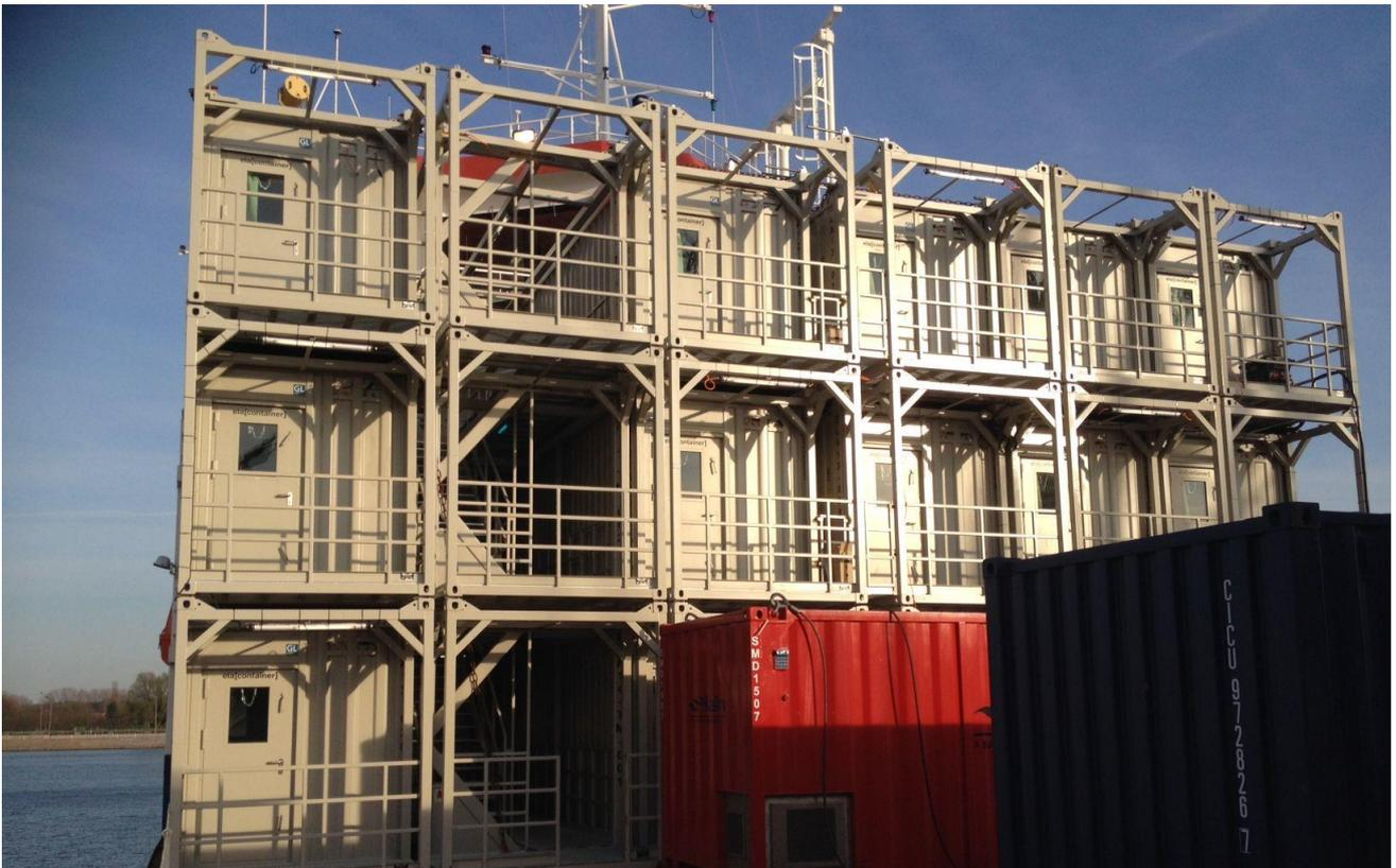
Offshore accommodation containers are not only needed on rigs and platforms but also for various types of ships: Three-story high container facility on a supply vessel
